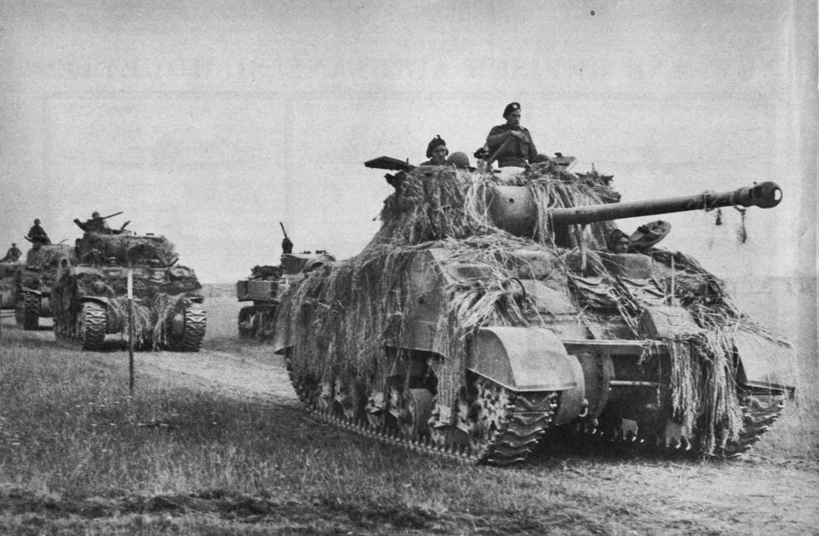
LONGEST-BARRELED GUN APPEARING ON THE U. S. M-4 TANK IS THE HIGH-VELOCITY 17-POUNDER RECENTLY INTRODUCED BY BRITISH IN NORMANDY
